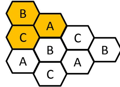
The  $N$  cells which collectively use the complete set of available frequencies is called a '**cluster**'. If a cluster is replicated ' $M$ ' times within the system, the total number of duplex channels,  $C$ , can be used as a measure of capacity and is given by
