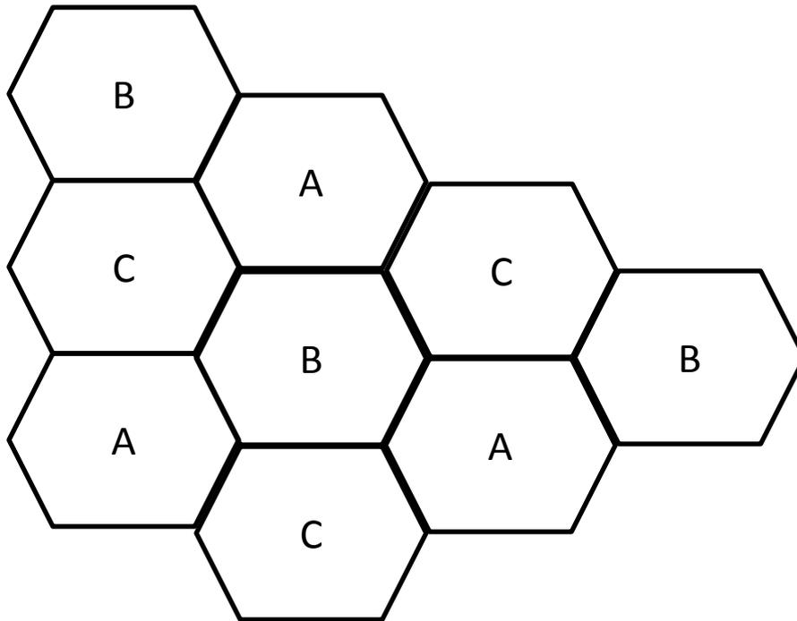
Illustration of a 3 cell cluster. In this case all the available channels are completely used up in 3 cells or *frequency reuse factor* =  $1/3$
